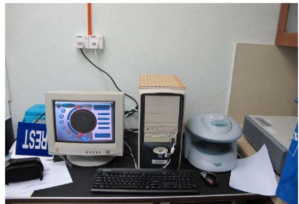
Figure 4: aCOLyte colony counter connected to the computer.
